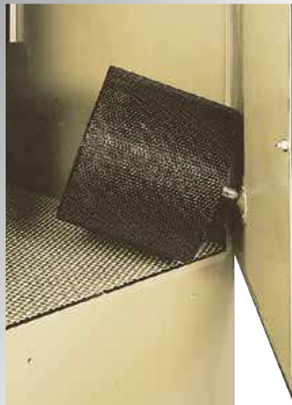
4.5 cubic-foot media storage hopper provides a large supply of abrasives to support up to four blast guns.
