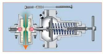
One reason for the popularity of SuperBlast® is our patented Sure-Flo® Media Regulator. The media path through the valve is straight down, assuring dependable flow. Abrasive media contacts only one part, a gumrubber metering tube. Not only is the tube exceptionally long lasting, it's also inexpensive and simple to replace, meaning you enjoy more productive time and virtually maintenance-free operation. Various metering tubes are available to match your application.
