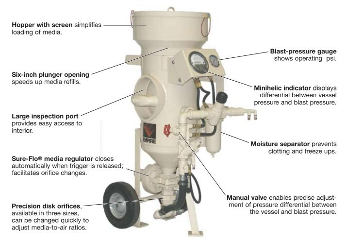
Empire SafeStrip™ portables are designed specifically to handle fine, light media used in the cleaning and stripping of delicate substrates. SafeStrip portables quickly and safely remove old coatings, dirt, oil, corrosion and other unwanted residues from soft metals, rubber, plastics and other sensitive surfaces. They are ideal for work on statues, monuments, machinery and molds, and in many other applications requiring a "light touch."
